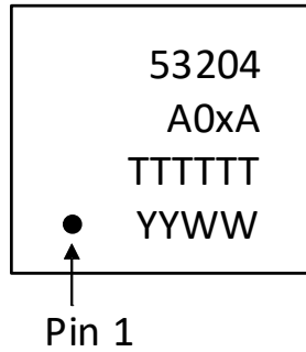
Figure 27. Si53204 Top Marking
