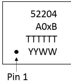
Figure 33. Si52204 Top Marking
