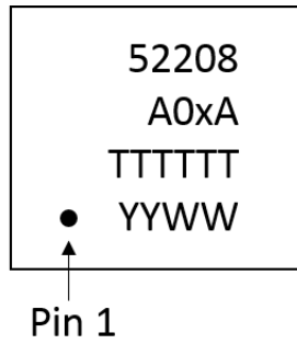
Figure 30. Si52208 Top Marking
