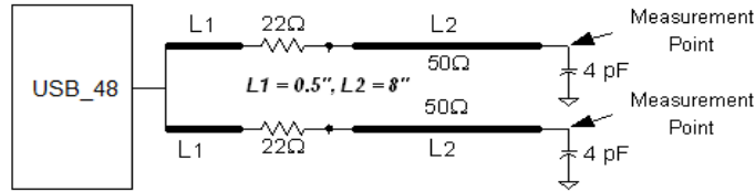
Figure 8. Single-ended USB_48 Clock Double Load Configuration
