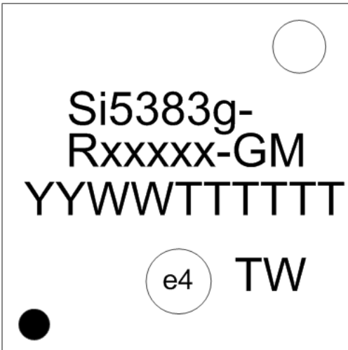
Figure 12.1. Si5383 Top Marking
