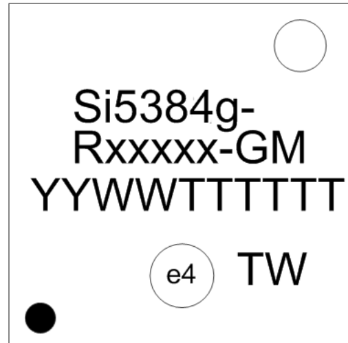
Figure 12.2. Si5384 Top Marking
