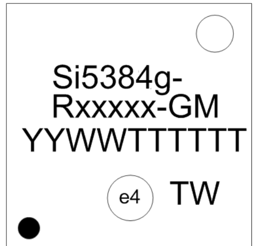
Figure 12.2. Si5384 Top Marking
