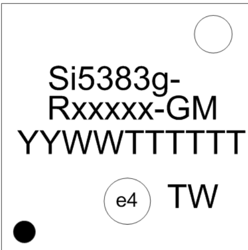
Figure 12.1. Si5383 Top Marking
