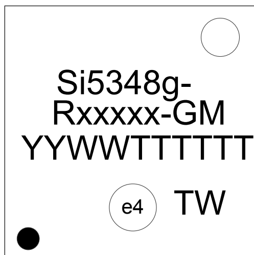
Figure 12.1. Si5348 Top Marking
