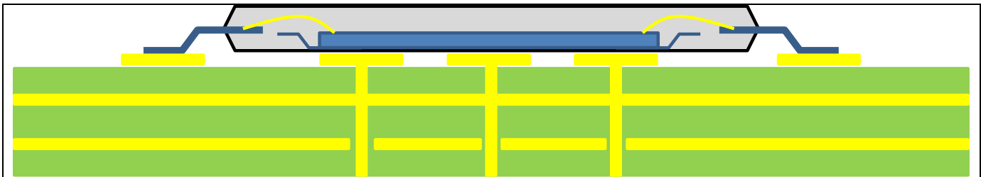
Figure 8-1: Example thermal via holes on PCB.
