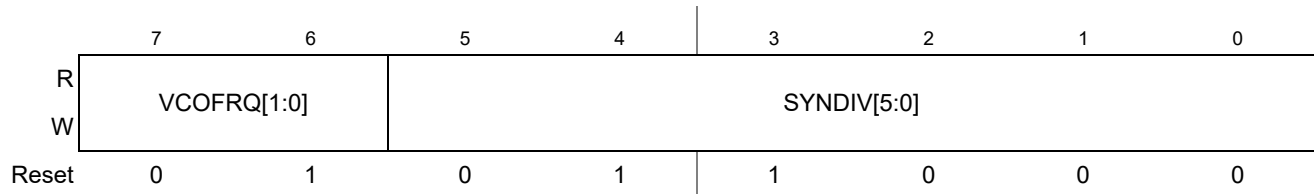
Figure 10-4. S12CPMU Synthesizer Register (CPMUSYNR)
