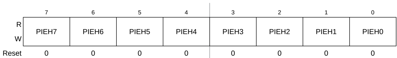
Figure 23-54. Port H Interrupt Enable Register (PIEH)
