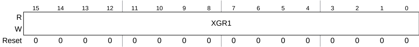
Figure 6-12. XGATE Register 1 (XGR1)
