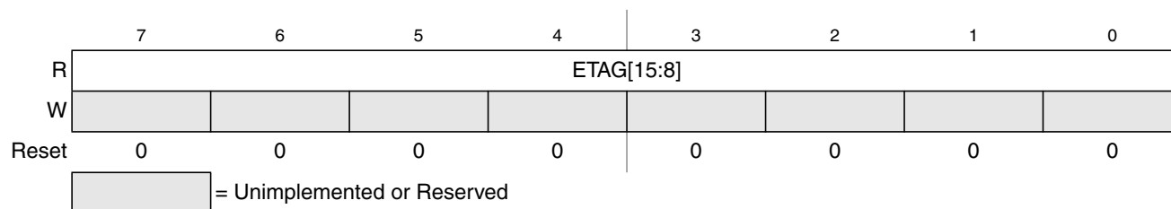
Figure 24-18. EEE Tag Counter High Register (ETAGHI)
