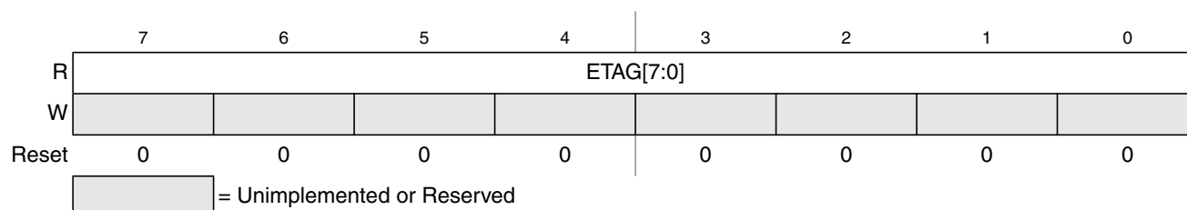
Figure 24-19. EEE Tag Counter Low Register (ETAGLO)
