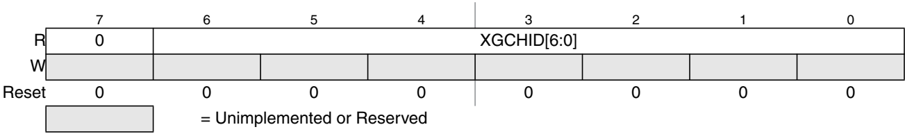
Figure 10-4. XGATE Channel ID Register (XGCHID)
