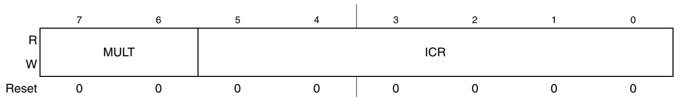
Figure 11-4. IIC Frequency Divider Register (IICF)
