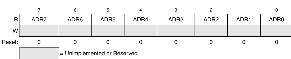
Figure 9-7. Data Result Low Register (ADCRL)
