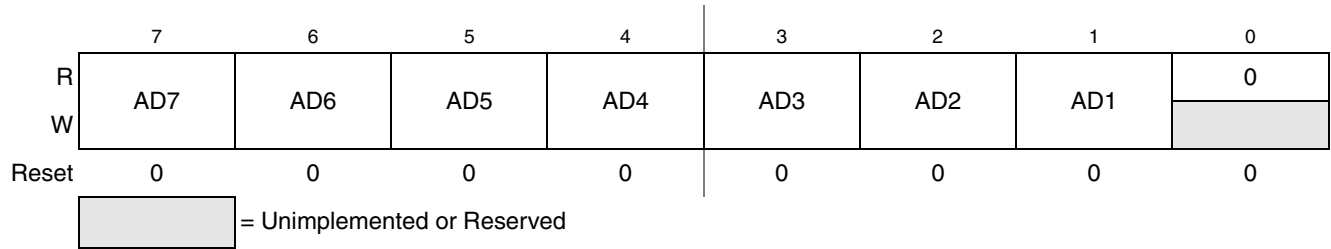
Figure 11-3. IIC Address Register (IICA)
