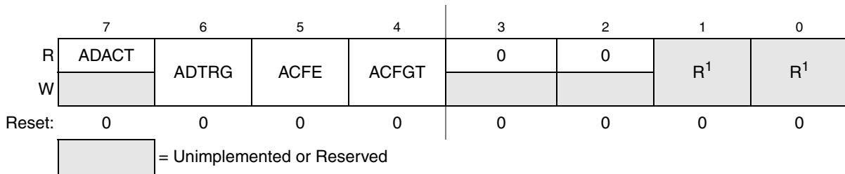
Figure 10-5. Status and Control Register 2 (ADCSC2)
