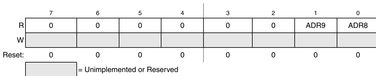
Figure 10-6. Data Result High Register (ADCRH)
