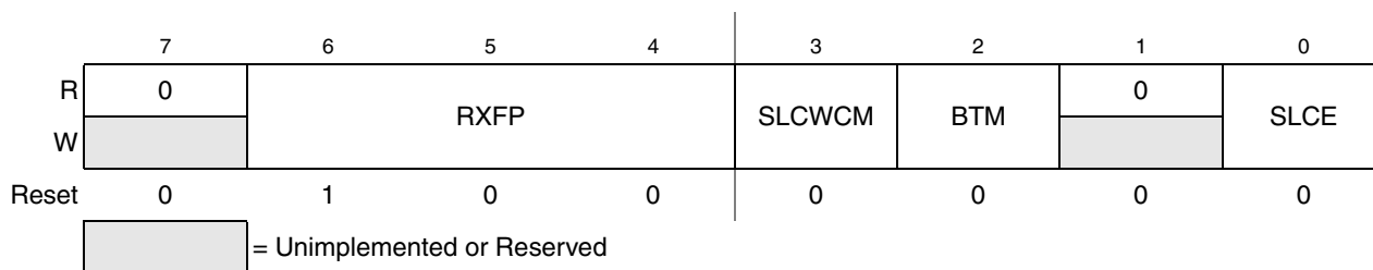
Figure 12-5. SLIC Control Register 2 (SLCC2)
