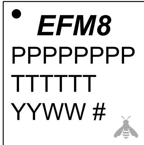
Figure 9.3. QFN32 Package Marking
