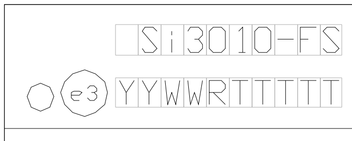
Figure 19. Si3010-F-FS Top Marking
