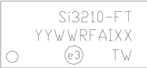
Figure 40. TSSOP Top Mark Diagram
