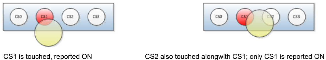
Figure 6. FSS when multiple buttons are touched with one button ON previously
