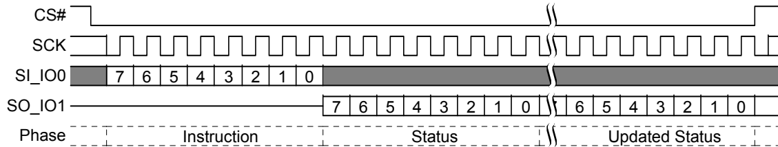
Figure 9.9 Read Status Register-1 (RDSR1) Command Sequence
