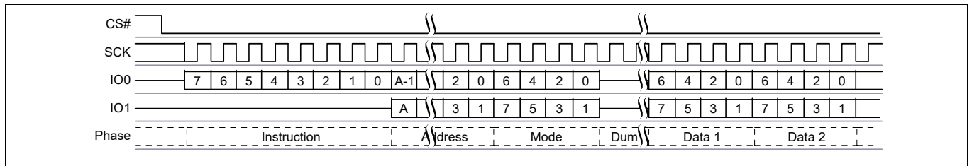
Figure 69 Dual I/O Read command sequence [32, 33]
