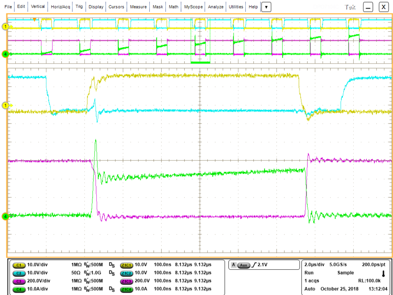
Figure 43. SiC MOSFET Switching Waveforms
