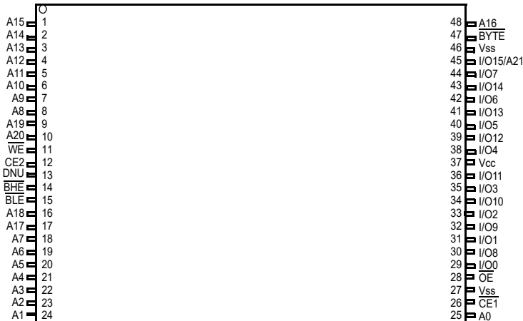
Figure 2. 48-ball FBGA pinout (Top View)
