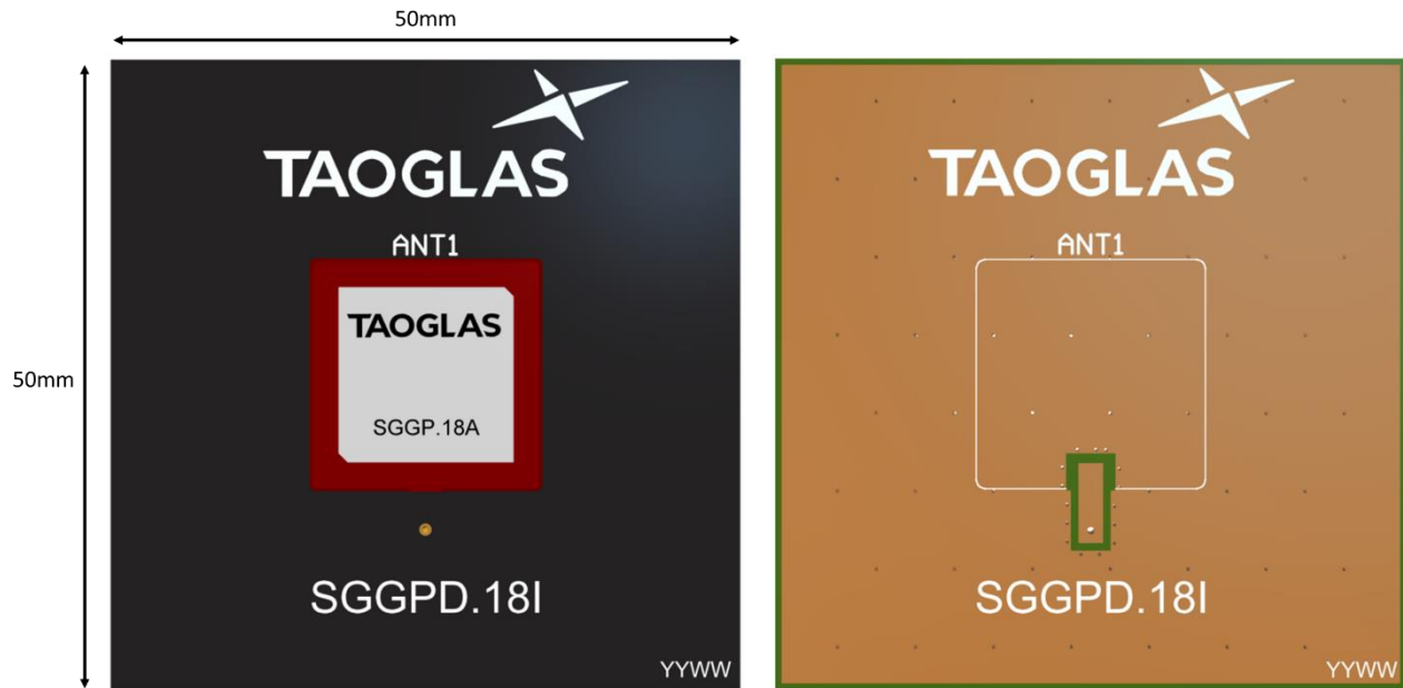
Top Side (SGGP.18.4.A.08 placement on 50x50mm PCB)
