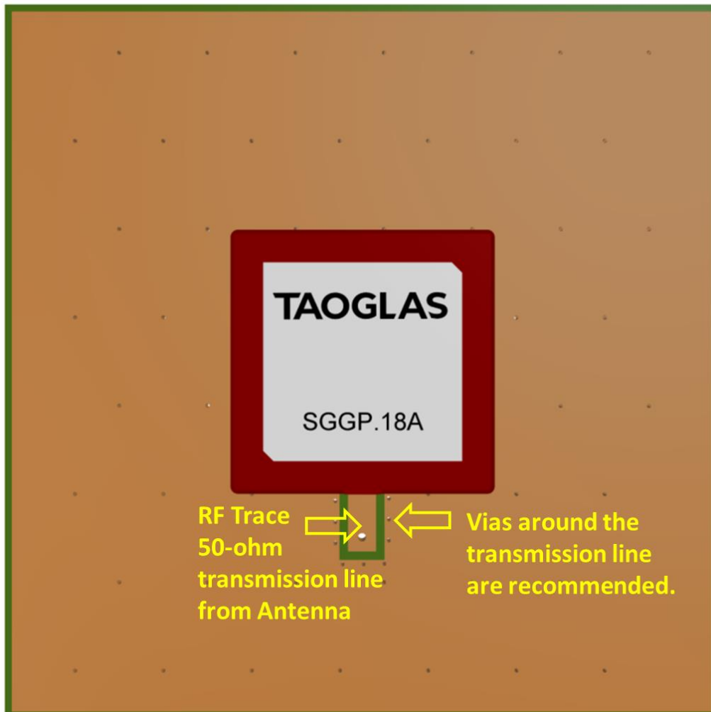
Top view of the PCB, showing transmission line and integration notes.
