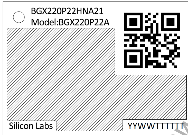
Figure 8.3. BGX220P Top Marking
