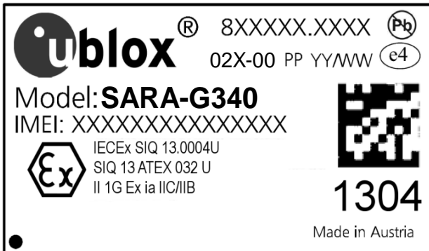
Figure 13: Label of SARA-G340 ATEX modules
