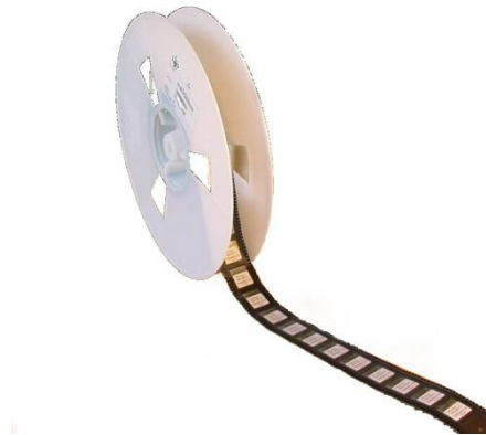
Figure 9: Reeled SARA-G3 series modules
