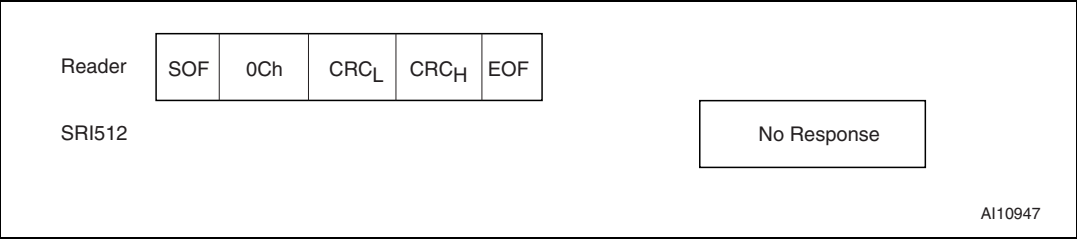
Figure 57. Reset_to_inventory frame exchange between reader and SRI512
