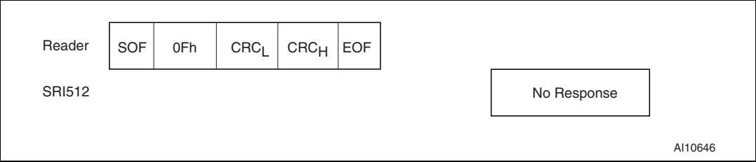
Figure 56. Completion frame exchange between reader and SRI512
