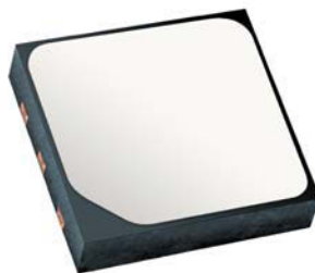
Figure 7. Si7021 with Factory-Installed Protective Cover
