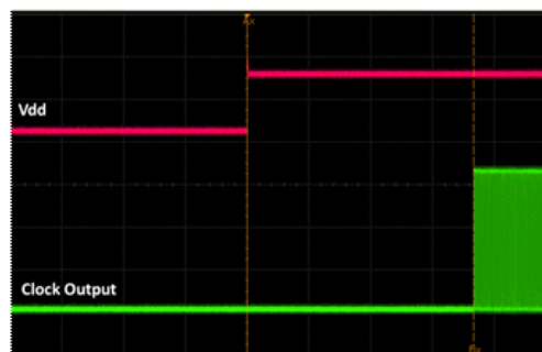
Figure 17. Startup Waveform vs. Vdd
