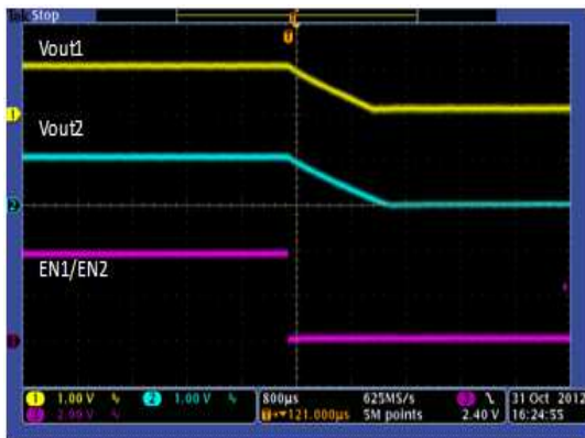
Figure 22. Shutdown With Enable
