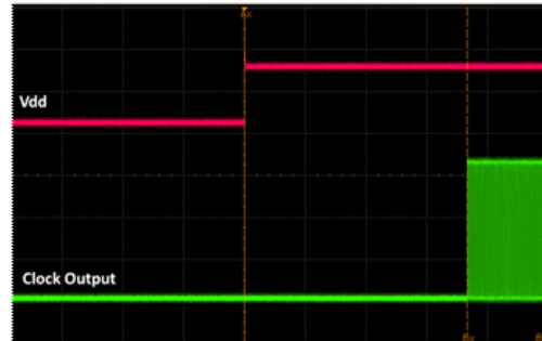
Figure 16. Startup Waveform vs. Vdd
