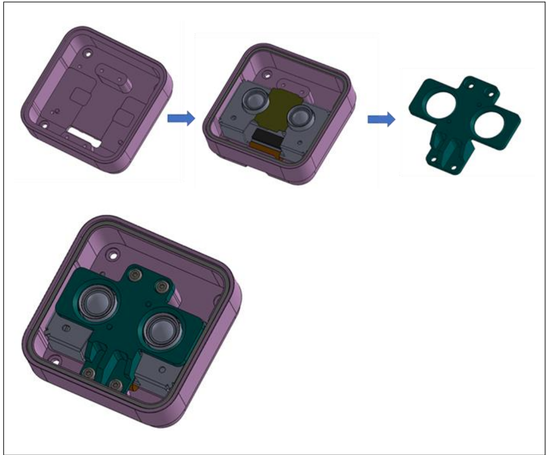
Figure 7-15. Stereo Depth Module Mid-Mounting – D401
