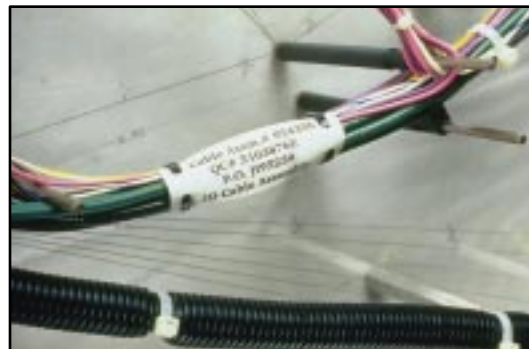
Identify harness board assemblies
