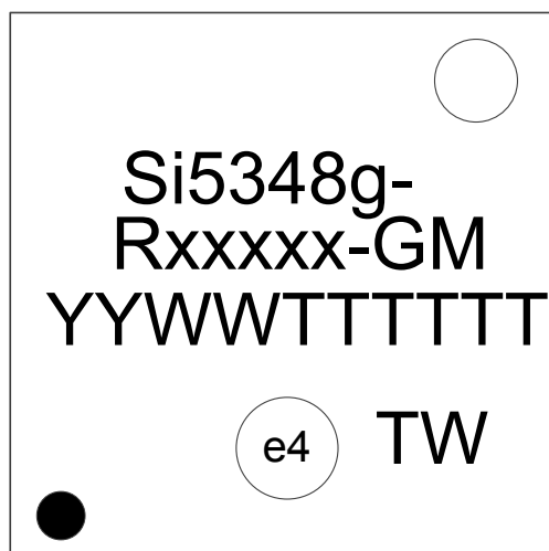
Figure 13.1. Si5348 Top Marking
