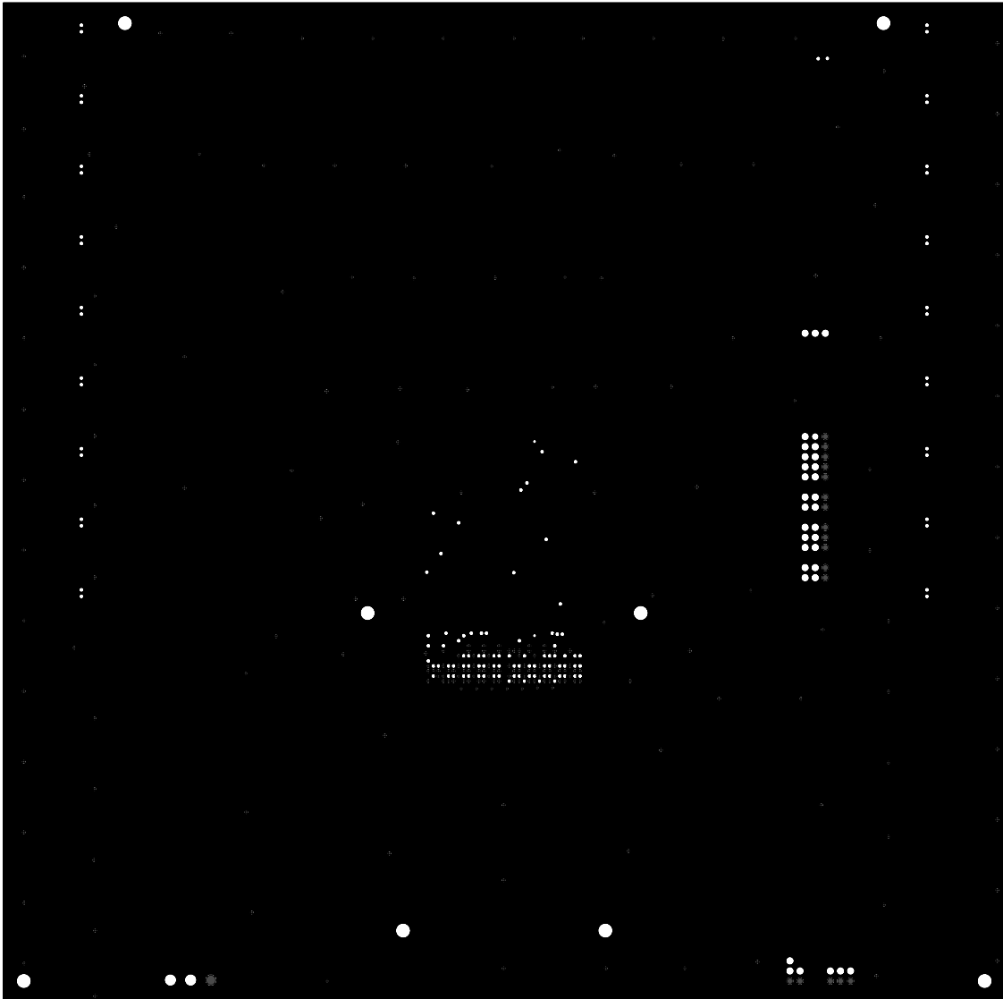
Figure 50. Layer 5—GND2 Plane (Optional Full-Duplex Motherboard)
