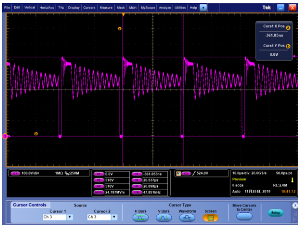
Figure 8-3 Max voltage of Vsw in DCM operation, V=100V/div, H=10µs/div, Vsw=518V/div, f=47.8 kHz
