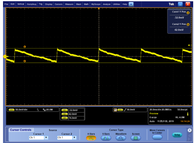
Figure 4-2 Vin=230Vac, V=50mV/div, H=20ms/div Vout ripple=74mVp-p, Pout=0W
