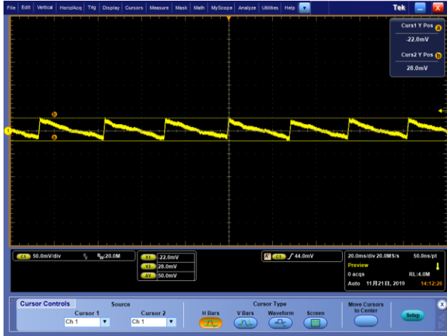
Figure 4-1 Vin=100Vac, V=50mV/div, H=20ms/div Vout ripple=50mVp-p, Pout=0W
