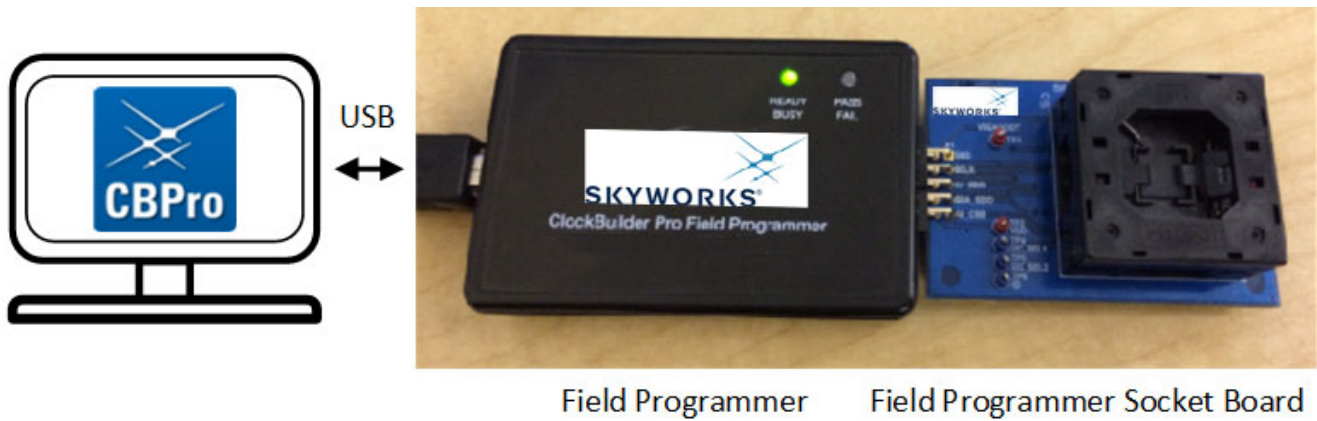
Figure 14. Connections from PC to the Target Device
