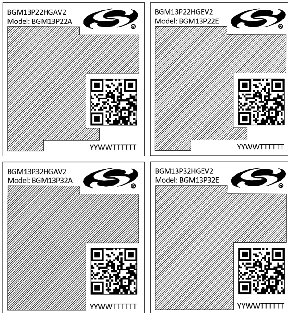
Figure 9.5. BGM13P Package Marking
