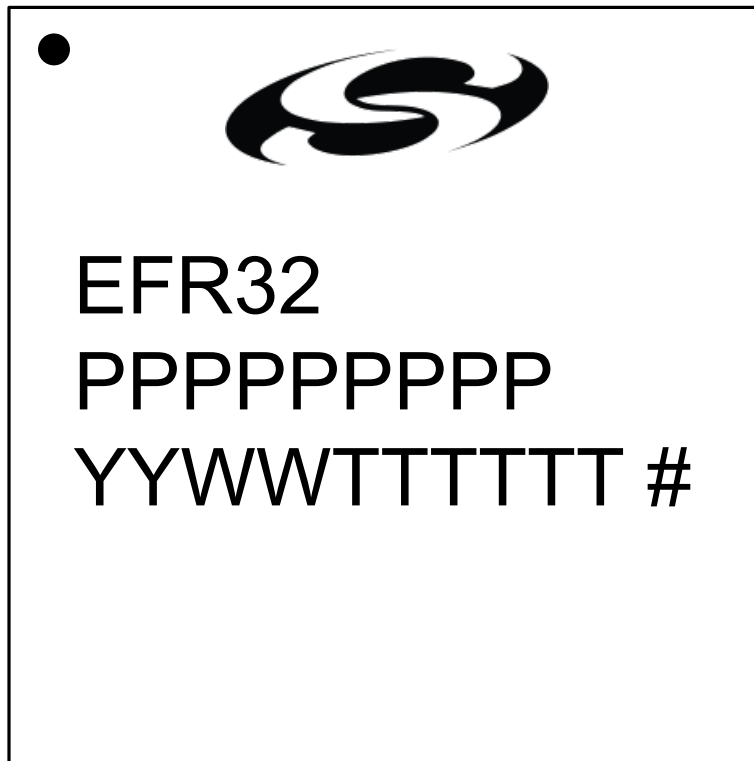
Figure 7.3. QFN48 Package Marking
