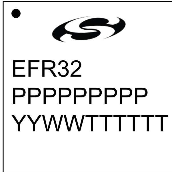
Figure 8.3. QFN32 Package Marking
