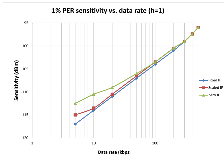
Figure 9. RX Architecture vs. Data Rate
