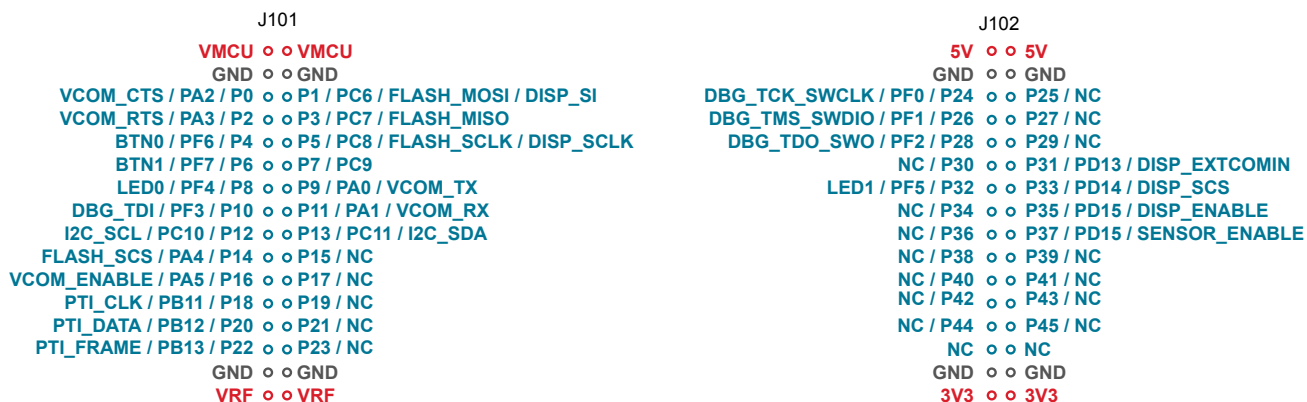
Figure 4.2. Radio Board Pin Mapping on Breakout Pads
