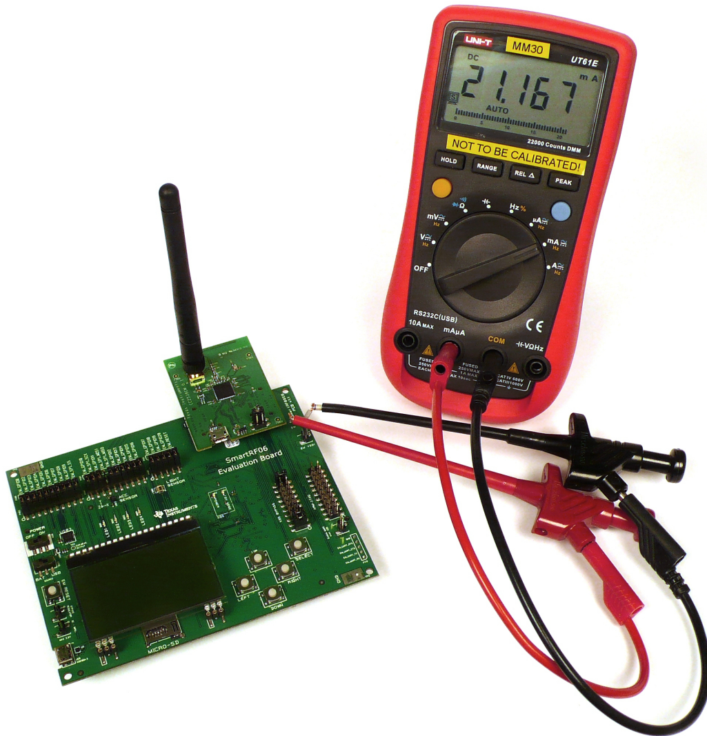
Figure 23. Measuring Current Consumption Using Jumper J503
