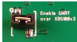
Figure 9. Jumper Mounted on J5 to Enable the UART Back Channel
