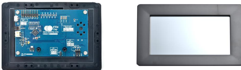
Figure 2-2 - VM801B module profile 5" display version
