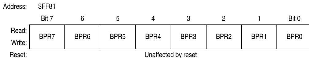
Figure 2-8. FLASH-2 Block Protect Register (FL2BPR)
