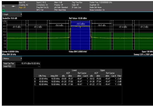
Figure 38. 20 MHz 802.11AC ACLR at 5825.0 MHz
