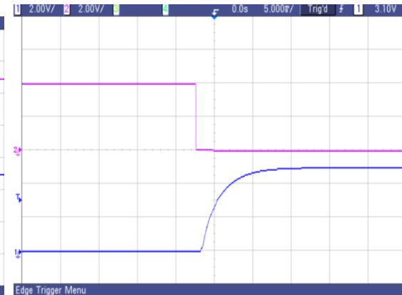
Fig.30 Typical start-up from CNT on of AVQ100B-48S05
