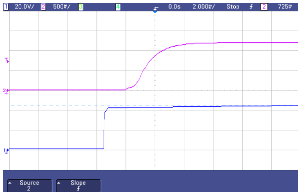
Fig.21 Typical start-up from power on of AGQ100-48S1V2
