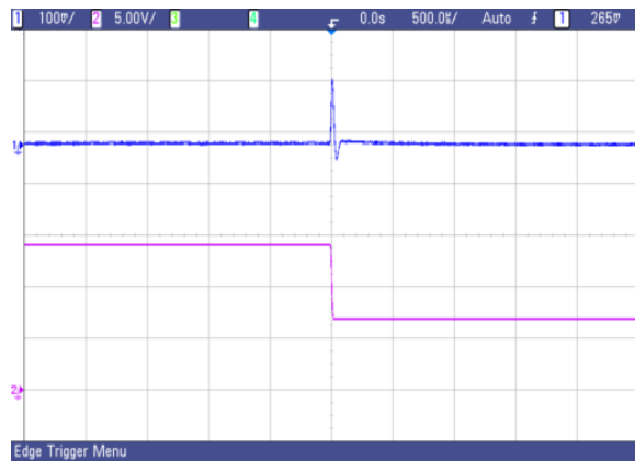
Fig.40 Typical transient response to step decrease in load from 50% to 25%, room temperature, 48Vdc input ( \Delta I_o/\Delta t = 1A/1\mu s ) of AVQ100B-48S05
