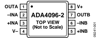
Figure 1. 8-Lead, MSOP (RM-8), ADA4096-2
