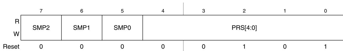
Figure 13-7. ATD Control Register 4 (ATDCTL4)
