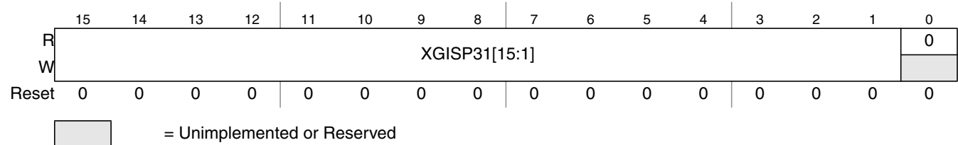
Figure 10-8. XGATE Initial Stack Pointer for Interrupt Priorities 3 to 1 (XGISP31)
