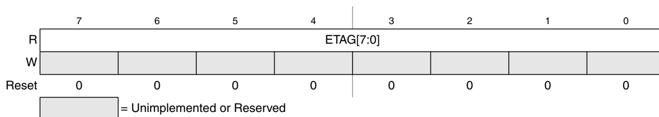
Figure 24-19. EEE Tag Counter Low Register (ETAGLO)
