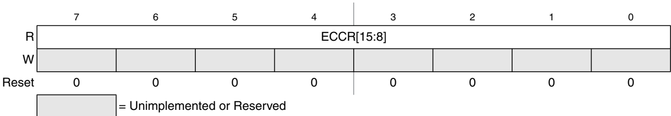
Figure 29-20. Flash ECC Error Results High Register (FECCRHI)
