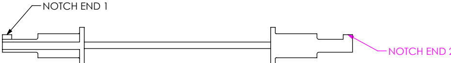
-NUS (END 2 NOTCH UP, CABLE STRAIGHT) (PIN 1 TO PIN N)
