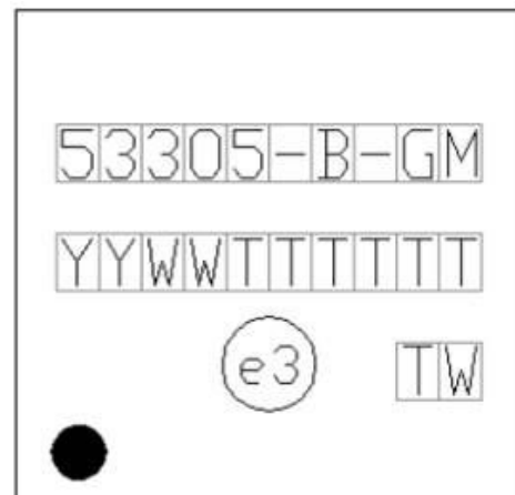
Figure 8.6. Si53305 Top Marking
