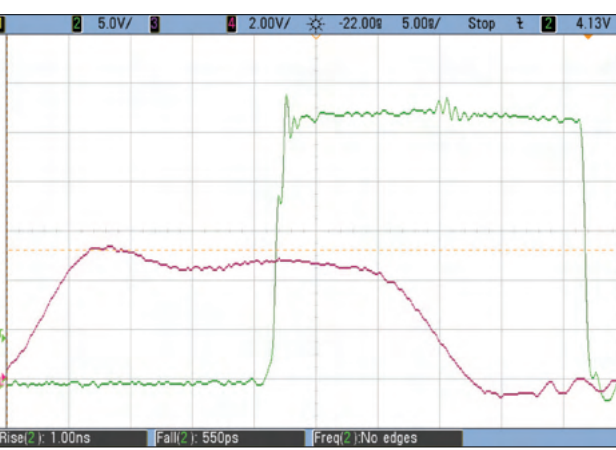
Figure 4: Typical Waveforms for V_{IN} = 28\text{ V} to 3.3 V/4 A (5 MHz) Buck converter CH2: ( V_{OUT} ) Switch node voltage — CH4: V_{PWM} Input voltage
