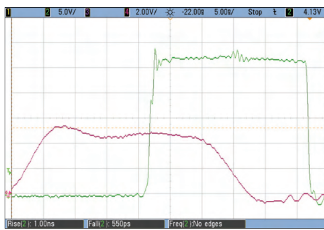
Figure 4: Typical Waveforms for VIN = 28 V to 3.3 V/4 A (5 MHz) Buck converter CH2: (V OUT ) Switch node voltage — CH4: V PM Input voltage
